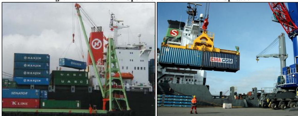
Fig. 5 A+B: Midstream Operation & Twin Lift Tower Spreader
