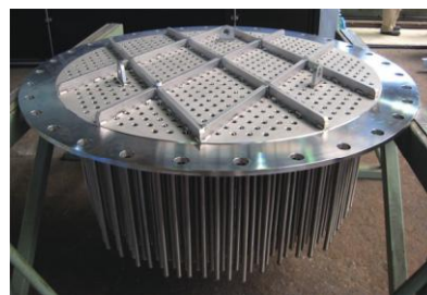
(b) Flange with its suspended spring filter
