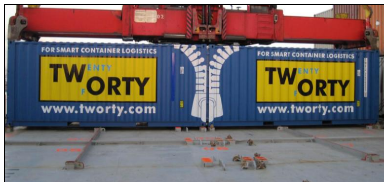
Fig 1. A pair of Tworty Boxes is loaded in coupled condition on board the "OOCL Montreal"
