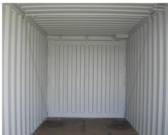
Fig 3. Inside view of closed additional front side door (cables to open the door are visible)
